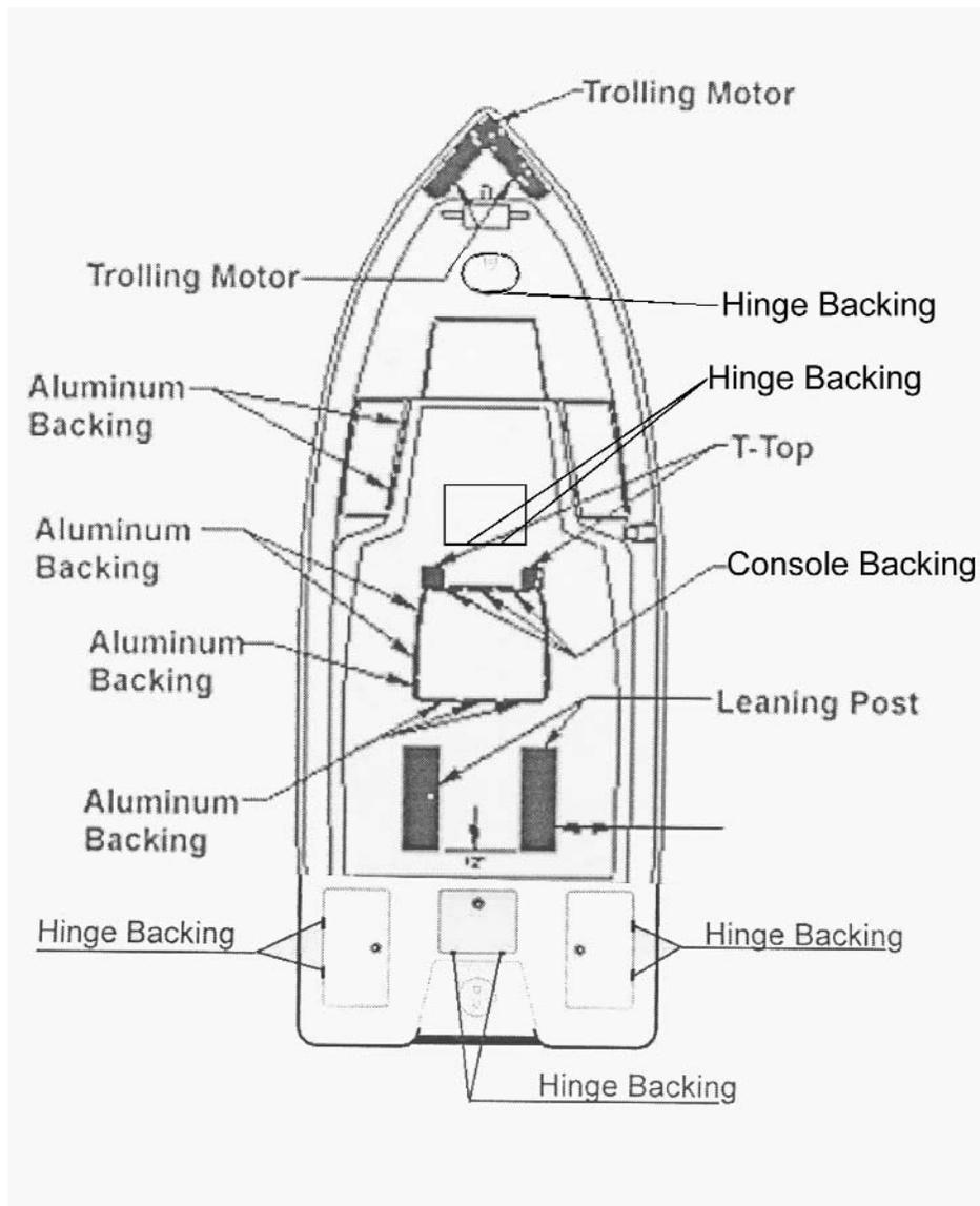
The above diagram shows all the aluminum backing plates (trolling motor, T-Top, Leaning Post) originally placed in the deck of a Pathfinder 2200-V Tournament Edition during the construction process. Other backing plates indicated are for hinge screw locations or to secure the console to the steering boss.
