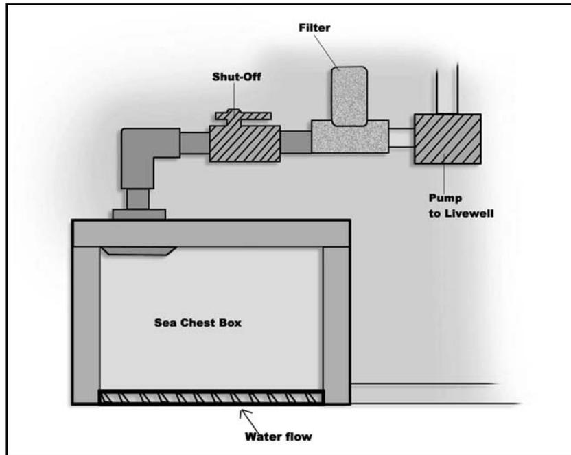
you turn your pump on, and water does not come into the livewell, check to make sure the filter is not clogged, thus preventing water flow into the system. To clean the filter, turn the shut-off valve to the 90-degree off position, unscrew the filter and pull out the screen.
