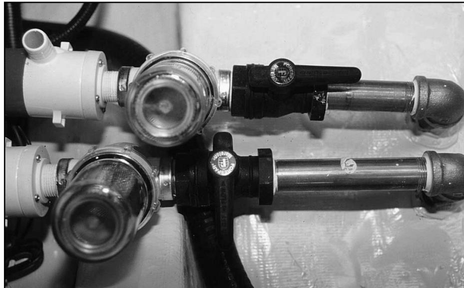
The livewell system at top is open and allows water to flow freely through the system. The lower livewell system is closed (90 degrees) to prevent water from entering.
