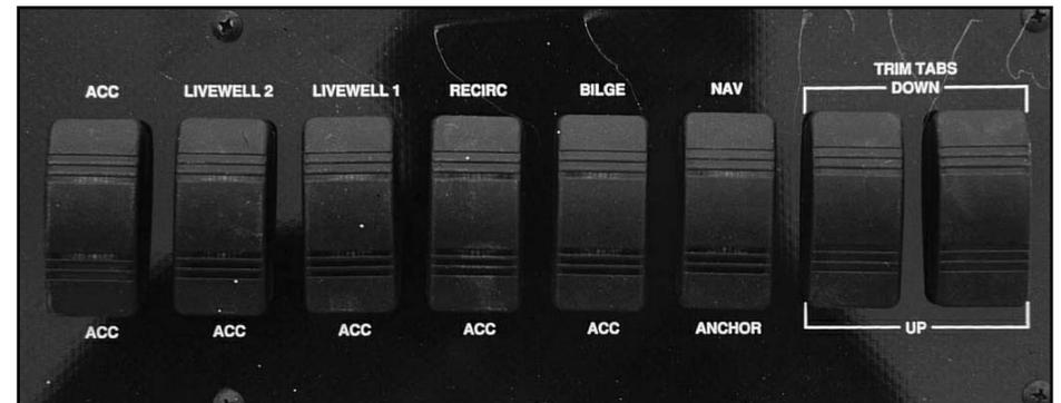
Shown above is the standard console switch panel for the Pathfinder 2200-V TE.
