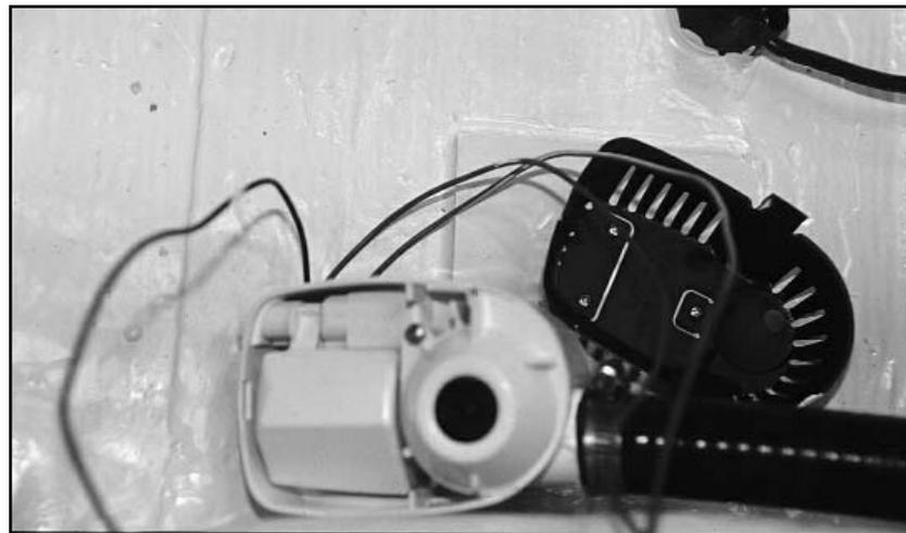
This bilge pump has been removed from its cradle and turned upside down. Inspect the impeller for clogs such as debris or small bits of monofilament.
